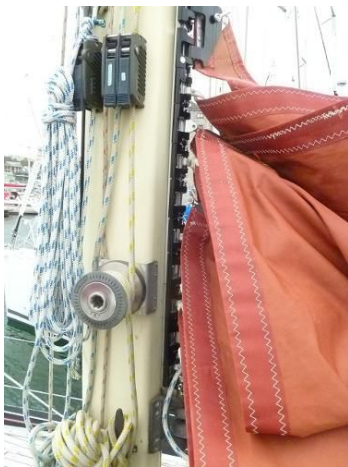
Low friction roller batten cars & luff track
