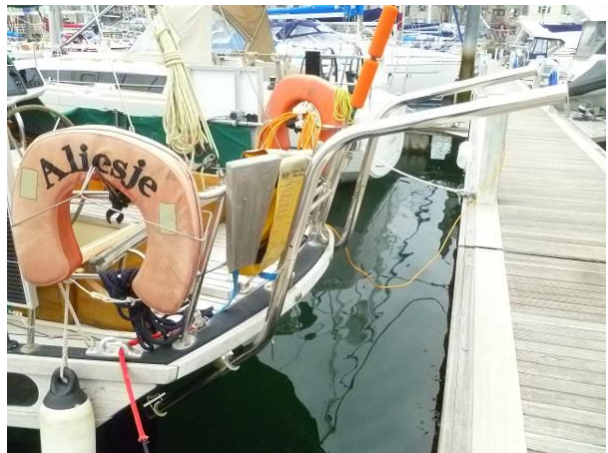
Stern davits - swivelling to reduce L.O.A
